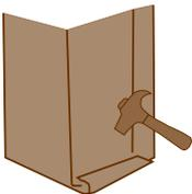
Neaten and flatten by using the hammer and pliers. Remove sharp edges
